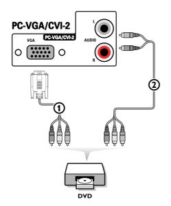
Connect the device with 2Fh YPbPr output to the VGA connector (1) (with the supplied adapter cable VGA to cinch) and to the L and R AUDIO jacks (2) of PC-VGA/CVI-2. See also the manual of your High Definition device.
