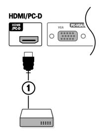
HDMI is the leading new standard for Digital High Definition video and audio interconnection. Eg. with a Digital Set top box, with HDMI-equipped devices like a DVD-R,AV receiver...
