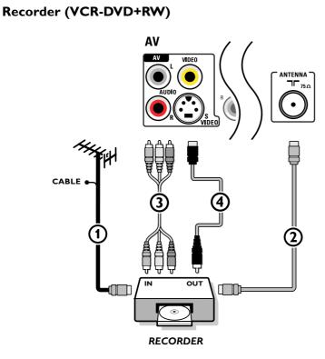
Note: Do not place your recorder too close to the screen as some recorders may be susceptible for signals from the display. Keep a minimum distance of 0,5m from the screen.
