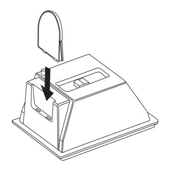
1 Lay down the main unit and then slide the base in the slot until it is fixed.
