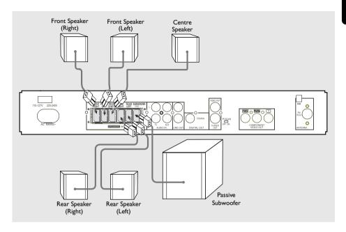
Connect the supplied speaker systems using the fixed speaker cables by matching the colours of the jacks and speaker cables.
