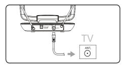
**3** Connect the DC plug to the antenna and the power supply to a 120V AC outlet.
