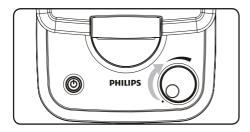
**3** Turn the TV or FM radio to the desired channel/station. Move the dipoles in different directions up and down until the reception is achieved.
