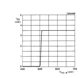
Fig.6 Keyed AGC output voltage  $I_{20}$  as a function of input voltage  $V_{14}$ . Measured in test circuit Fig.1 at  $V_3 = 2 \text{ V}$ ;  $V_{20} = 8.5 \text{ V}$ .
