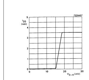
Fig.5 Keyed AGC output current  $I_{20}$  as a function of RMS input voltage  $V_3$ . Measured in test circuit Fig.1 at  $V_{14} = 0.7$  V;  $V_{20} = 8.5$  V.
