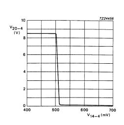
Fig.4 Keyed AGC output voltage  $V_{20}$  as a function of input voltage  $V_{14}$ . Measured in test circuit Fig.1 at  $V_3 = 2$  V;  $I_{20} = 0$ .
