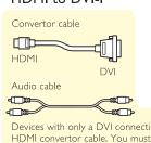
Devices with only a DVI connection can be connected with a DVI to HDMI convertor cable. You must connect the Right(Red) and Left(White) audio connectors of AVI of the TV to the audio output connectors of the device. Go to menu => Setup => Source => Analog Audio In => and select HDMI.
