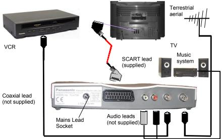
**Note:** When connecting SCART cable please ensure you follow indications on cable. Light grey end connected to DCB and black end connected to TV/VCR.
