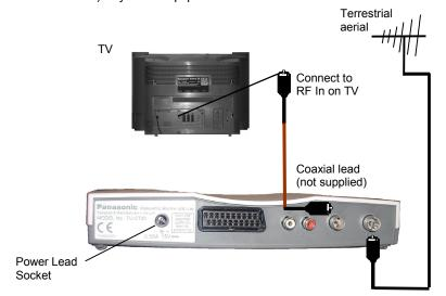
Connection of DCB and VCR using Scart and RF cables
