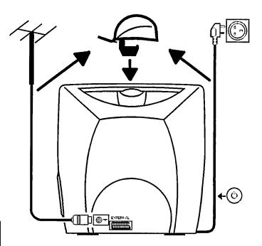
1 Insert the aerial plug into the socket.
