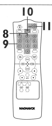
Turn off the VCR for the recording. Insert a tape in the VCR.
