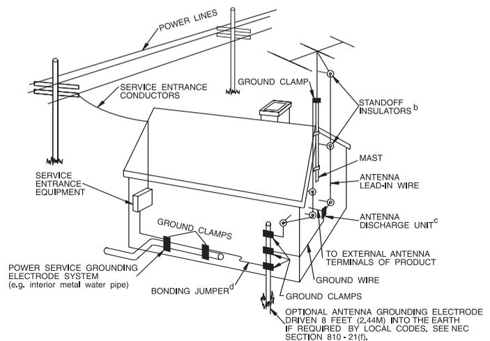
provide some protection against voltage surges and built-up static charges.
