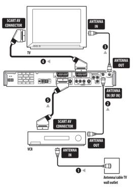
1 Connect the cable from the antenna/cable TV outlet to the antenna input on your VCR.
