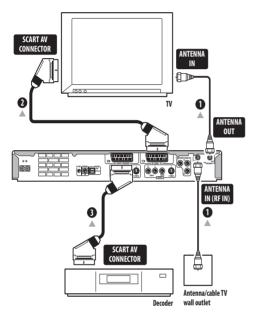
1 Connect RF antenna cables as shown.
