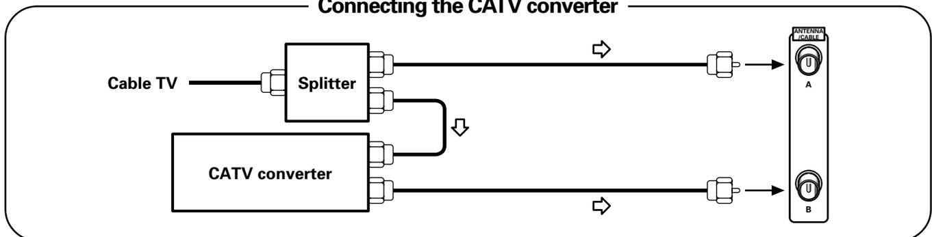
Connecting the CATV converter with VCR
