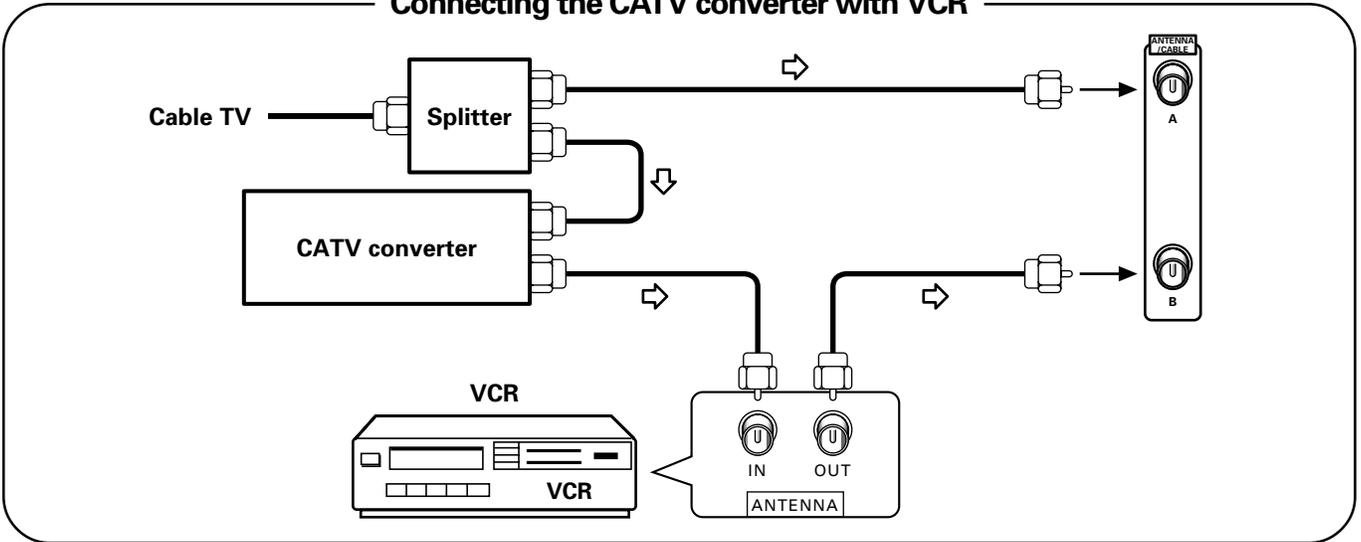
Connecting VHF/UHF antenna and CATV converter
