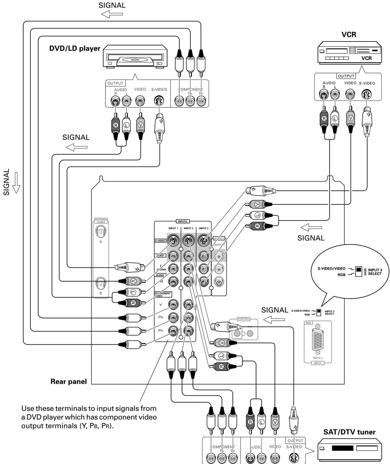
Use these terminals to input signals from a DVD player which has component video output terminals (Y, Pb, Pr).
