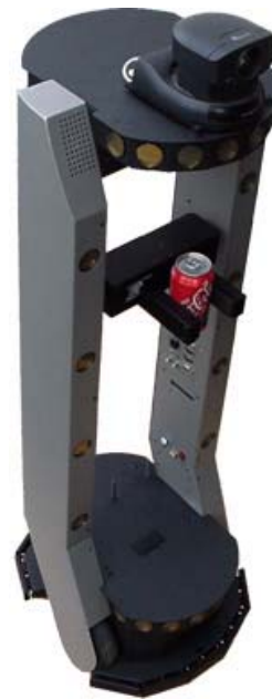
Figure 6. The Performance PeopleBot sports an attractive body design and bundled systems, including voice synthesis and recognition for human-interaction research and applications.
