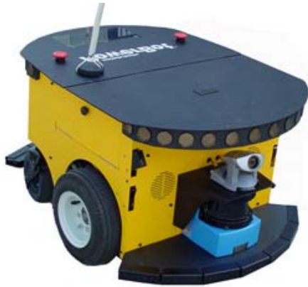
Figure 7. PowerBot carries over 100 ka of payload.
