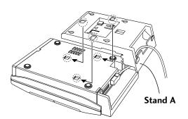
• If you have the optional cassette deck, MD recorder or CD-Recorder, connect these before attaching Stand A. (The ribbon cable can pass under the Stand A to keep it tidy.)
