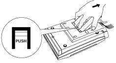
• To remove Stand A, pull the tab, as indicated, and slide off.
