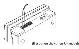
For best results, extend the FM antenna fully and fix to a wall or door frame. Don't drape loosely or leave it coiled up. The supplied FM antenna is a simple means of receiving FM stations; using a dedicated, outdoor FM antenna will usually give you better reception and sound quality. See below for connection details.
