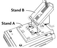
• To remove Stand B, push the center tab, as indicated, and slide off.
