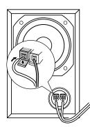
**3 Connect the other end to the amplifier.** The cable will only plug in one way; line up the plug and socket before fully inserting.
