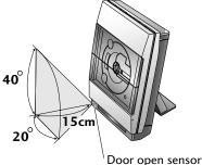
On its default setting, the door open sensor may open the disc compartment even if a CD is playing. You can change this so that it will only work if the CD player is stopped, or you can switch it off altogether (see page 36).
