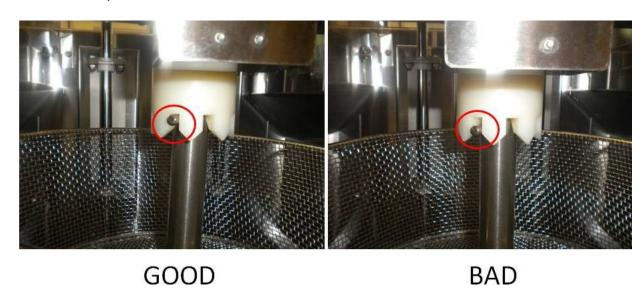
Check to assure that the top plate springs are not extending while the basket drive pin is in the coupling.
