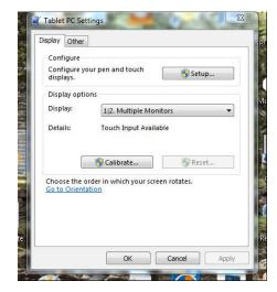
When you click on Calibrate, a grid pattern shows on the screen with touch points identified. Touch all of the identified points, then hit "yes" at the end to store the calibration.
