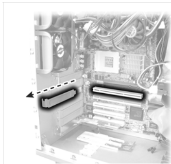
Use an available PCI or PCI Express slot.
