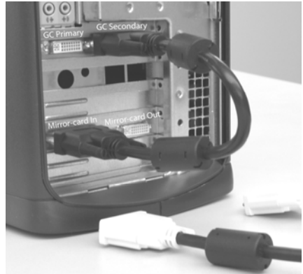
Short DVI cable installed
