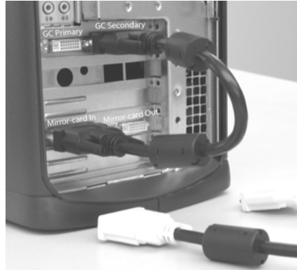
Short DVI cable installed
