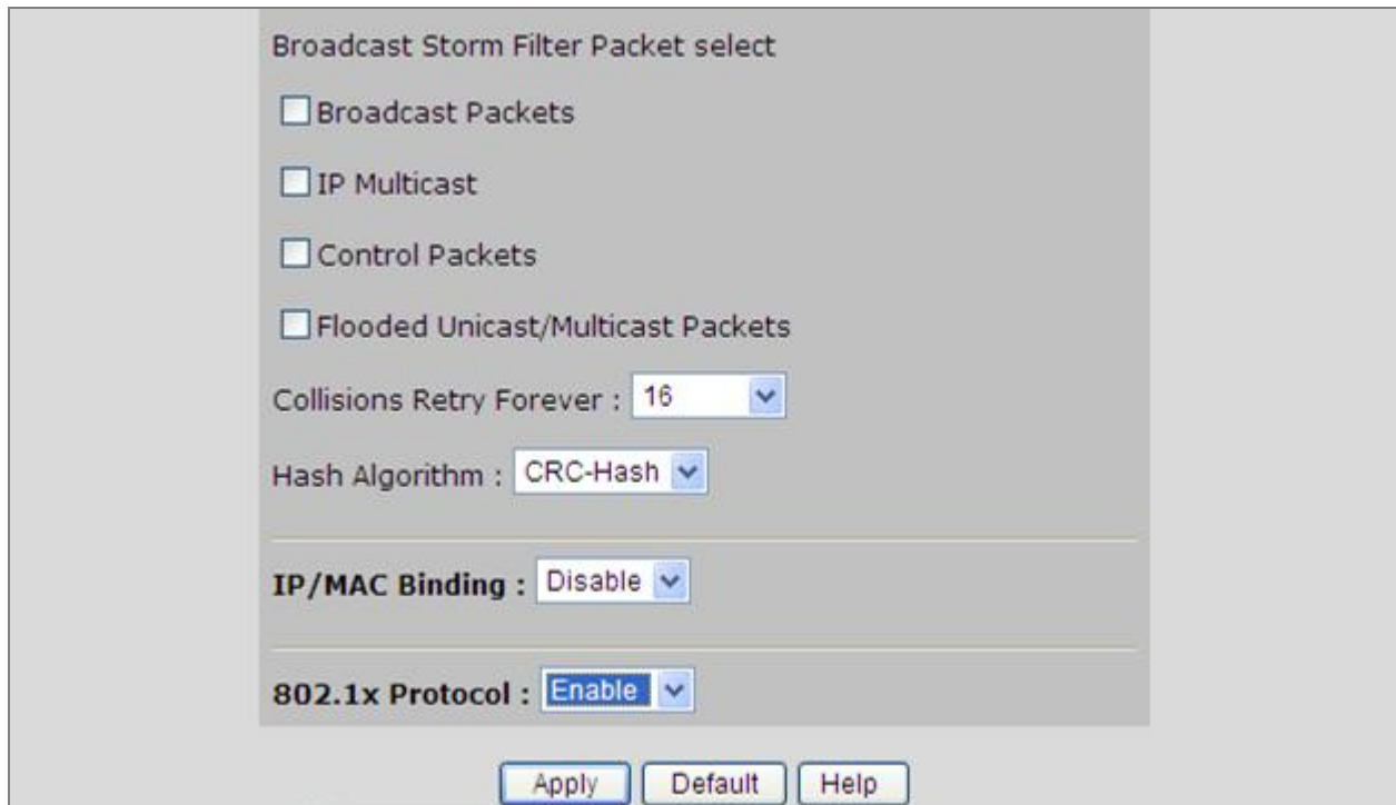
Figure 4-12-3: System information \ Misc Configuration \ 802.1x Protocol
