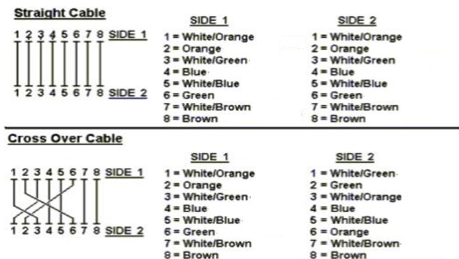
Figure A-1: Straight-Through and Crossover Cable
