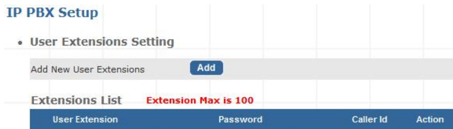
Figure D-3. User extension setting of IP PBX
