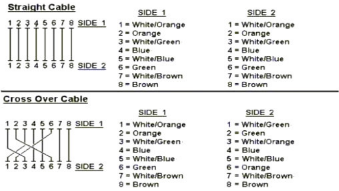
Figure A-1: Straight-Through and Crossover Cable
