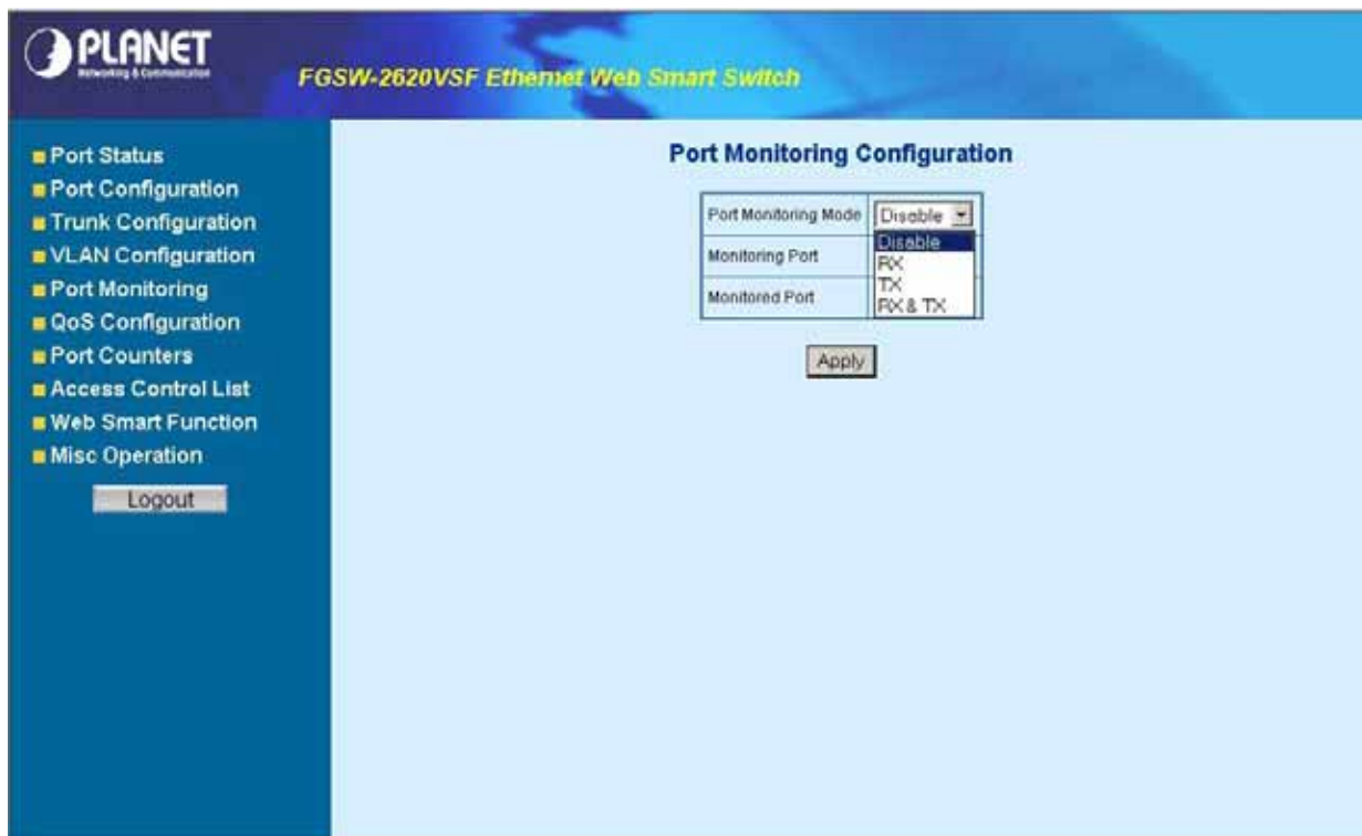
Figure 4-28 Port Monitoring Web Page screen
