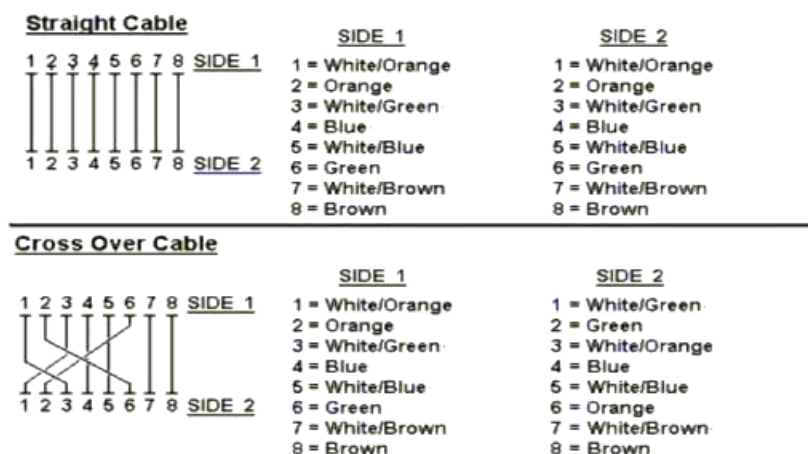
Figure A-1: Straight-Through and Crossover Cable
