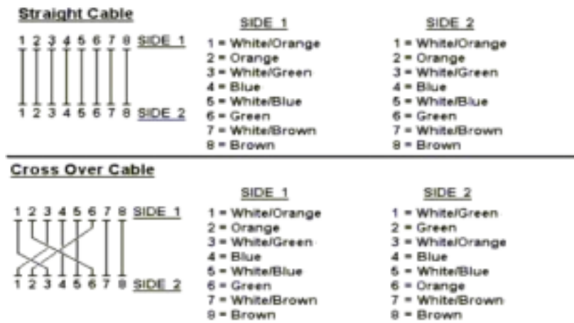
Figure A-1: Straight-Through and Crossover Cable
