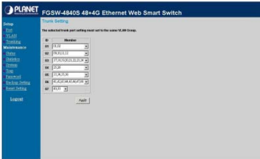
Figure 3-35 Trunking Setting screen
