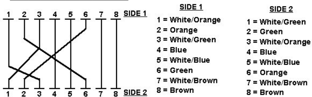
Figure A-1: Straight-Through and Crossover Cable
