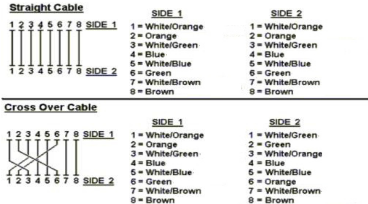
Figure A-1: Straight-Through and Crossover Cable
