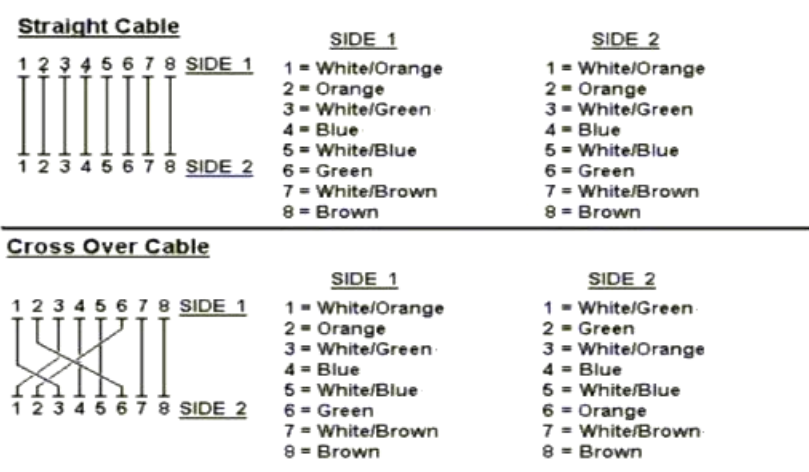
Figure A-1: Straight-Through and Crossover Cable
