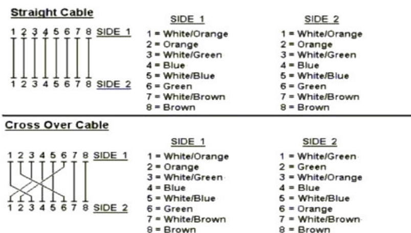
Figure A-1: Straight-Through and Crossover Cable
