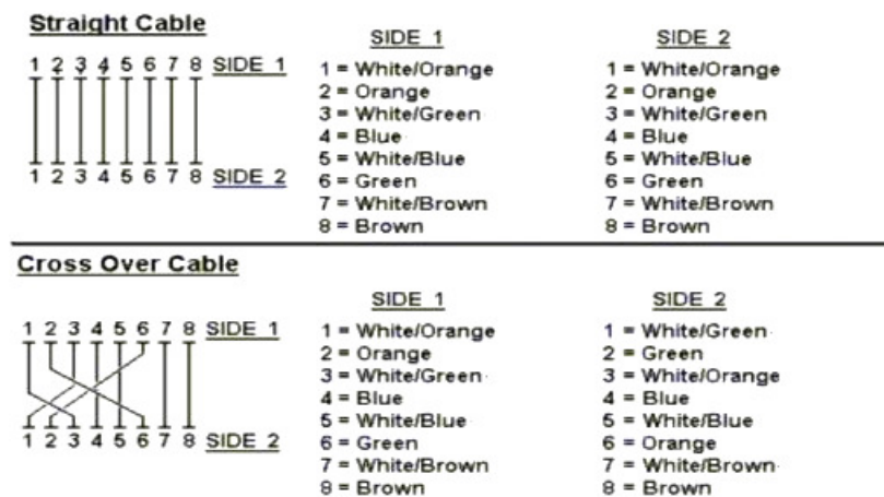
Figure A-1: Straight-Through and Crossover Cable
