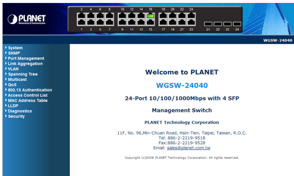
Figure 6-3 Web Main Screen of WGSW / SGSW Managed Switch
