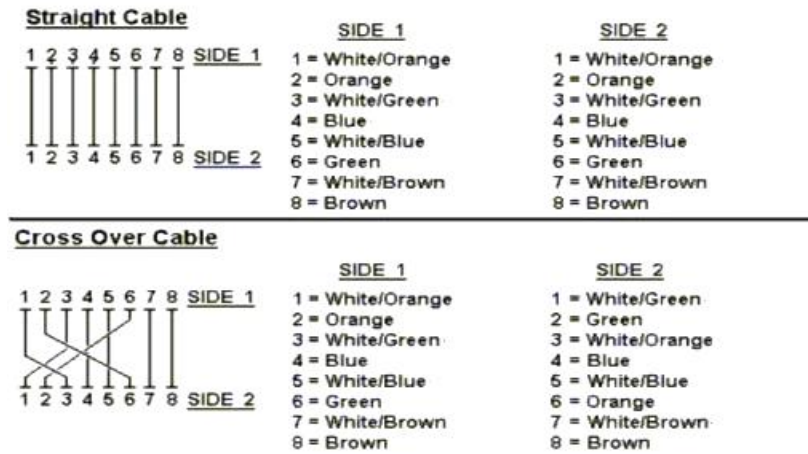
Figure A-1: Straight-Through and Crossover Cable
