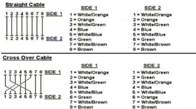
Figure A-1 Straight-Through and Crossover Cable
