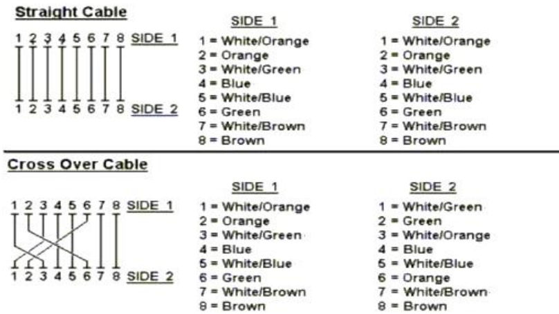
Figure A-1: Straight-Through and Crossover Cable
