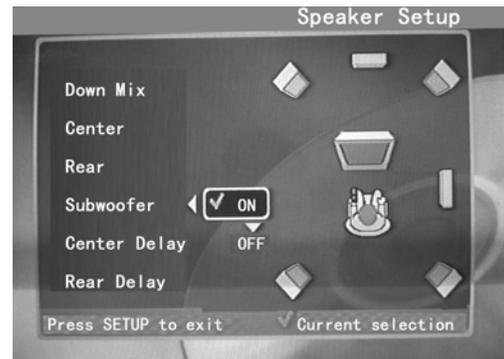
Figure 7. Activating The Center, Rear and Subwoofer Speakers
