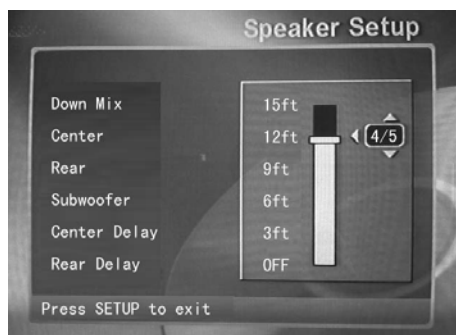
Figure 7. Establishing Center and Rear Speaker Delays
