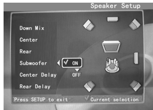
Figure 6. Activating The Center, Rear and Subwoofer Speakers
