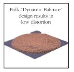
Laser Interferometry tests produced holographic "photos" of drivers in motion. The "bad" drivers are experiencing modal breakup that results in performance-robbing resonances. A "perfect" driver would look like a cake (flat on top), more, like the photo on the right.
