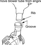
Insert the elbow tube into the blower outlet. Make sure elbow tube rib is aligned with the blower outlet groove.
