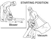
WARNING: When starting engine, hold the unit as illustrated. Do not set unit on any **WARNING:** surface except a clean, hard area when starting engine or while engine is running. Debris such as gravel, sand, dust, grass, etc. could be picked up by the air intake and thrown out through the discharge opening, damaging the unit or property, or causing serious injury to bystanders or the operator.
