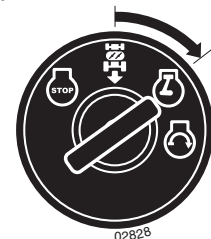
ENGINE "ON" POSITION (NORMAL OPERATING)
