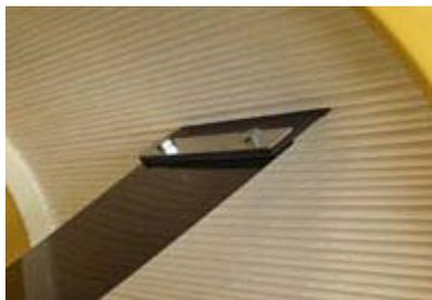
To help maintain the filtering efficiency a pair of hands (left) wipe across the inside of the pleated canister element to knock off excess buildup. The hands are operated by a simple turn of the exterior handle (right). Giving the handle a single turn once per month is adequate in most situations.
