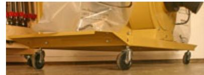
Full swivel casters at each corner of the solid metal base make moving the DC1900 around the shop safe and easy.
