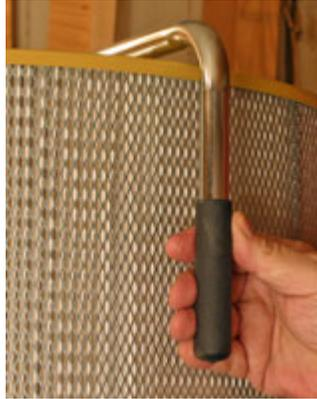
A pair of "hands" (left) within the canister flex the pleated element to knock off excess buildup. The hands are operated by the external handle (right), which is generally turned through one revolution per month in most home woodshop circumstances.
