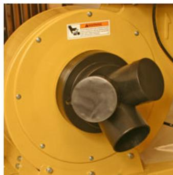
The inlet ports are mounted directly to the blower housing, putting them low on the POWERMATIC PM1900 and on an even plane with the dust outlets on many machines. This alignment keeps more of the hose flat on the floor for safety and eliminates much of the lifting loss higher inlet ports experience to enhance performance.
