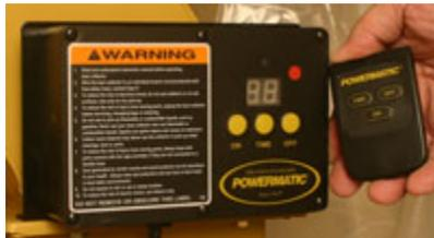
The infrared remote (1Ph version only) can save untold steps back and forth to the DC1900. It also has a timer function that allows programming in up to 99 minutes of run time before the DC1900 shuts off automatically.
