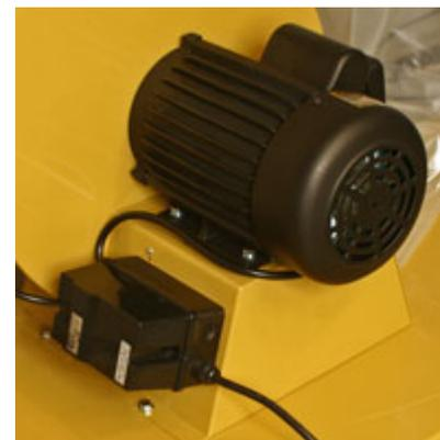
The 3 HP motor (1Ph version only) features a magnetic start switch that protects the motor itself, and you from unexpected power variations or outages.
