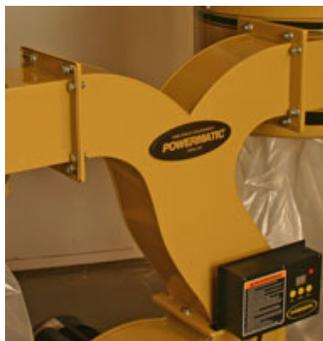
The smooth surfaces and curves of the sheet metal chute (left) enhance airflow and efficiency. This triple 4"-outlet adapter (right) slips onto an 8"-diameter port to provide the most versatility in your shop.
