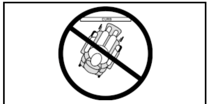
Figure 3. Incorrect Curb Approach
