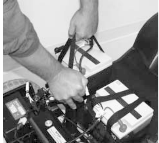
Figure 19. Put Batteries in Place
