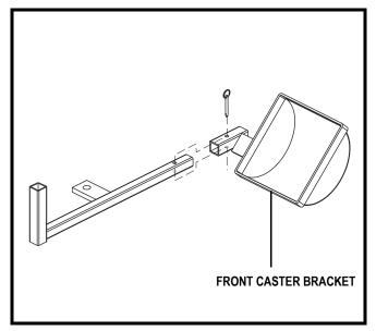
3. Install the front caster bracket and secure with the detent pin.
