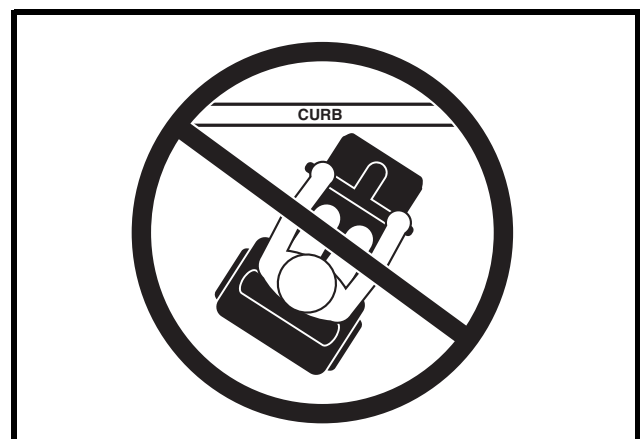
Figure 3A. Incorrect Curb Approach
