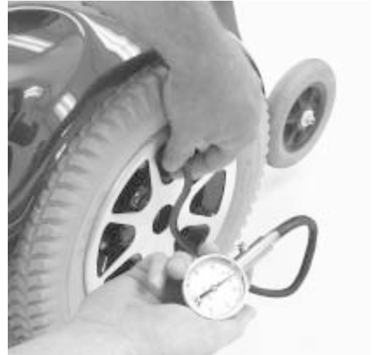
Figure 38. Check Tire Pressure
