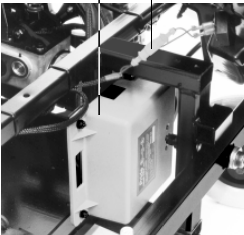
Figure 26. Onboard Battery Charger
