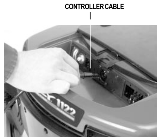
Figure 11. Controller Cable Connection
