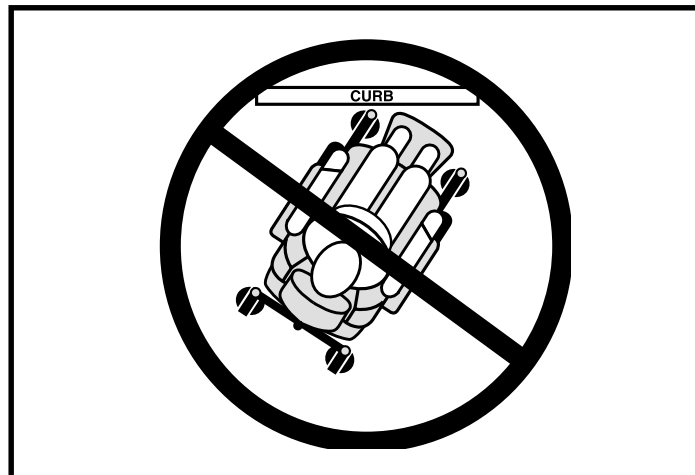
Figure 3. Incorrect Curb Approach
