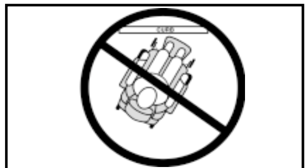
Figure 3. Incorrect Curb Approach
