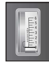
Figure 8. Ammeter Indicates Battery Is Fully Charged
